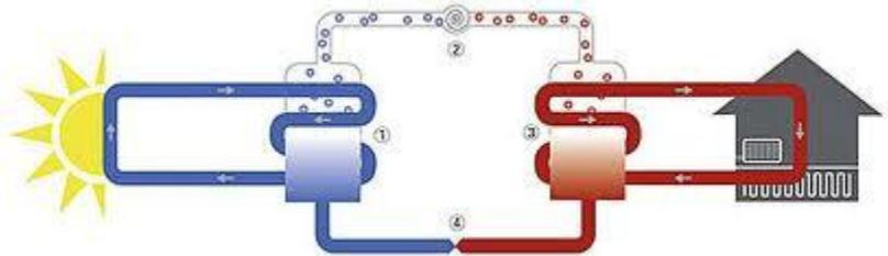
As a rule of thumb, for every degree we can increase the energy source temperature entering the heat pump, it will improve the heat pump performance by approximately 2% and for every degree that we can reduce the energy supply requirement in the occupied space we improve energy efficiency by approximately 1 ½%.
